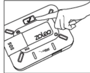
While the message is being sent, each LED will emit a green flash in turn. An ascending tone is emitted when the message has been sent. If less than the minimum allowable time between check-in messages has elapsed (i.e. 2 minutes), the check-in message will fail, and the device will emit a descending tone. The ZOLEO App will show a check-in countdown displaying when your next available check-in window commences. Once sent, a check-in message cannot be cancelled.
